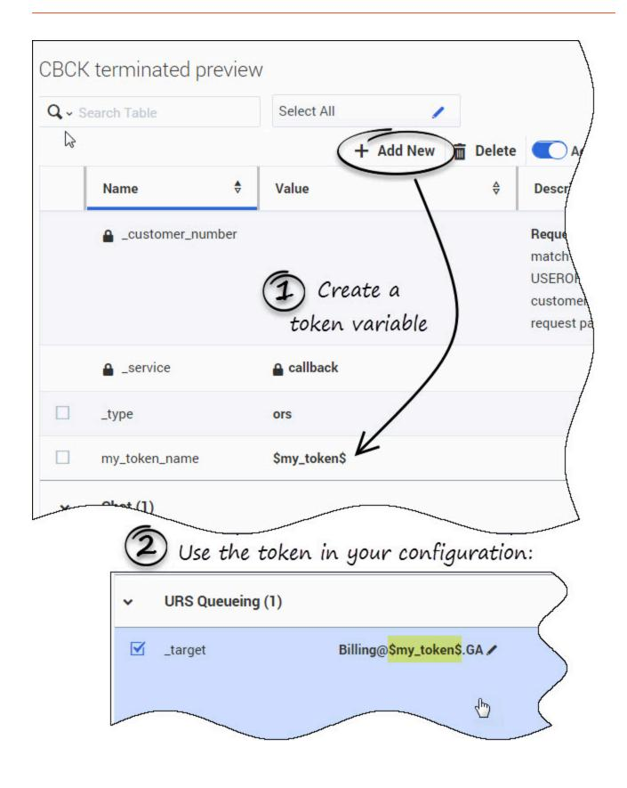
To create a token variable, create a new service parameter and configure its value with a string matching the following format: \$<any-token-name>\$
