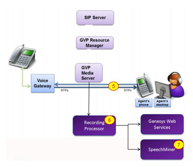
When the recording ends, SIP Server re-invites the session to have media sent directly between the parties. Media Server submits the recording to storage and to the Recording Processor (5).
