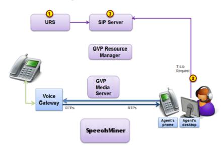
There are three ways that recording can be initiated. Once started, the recording process is the same, regardless of how it was initiated.
