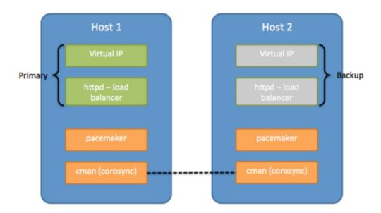
As a simple two host primary/backup solution, the hosts must be deployed on the same subnet that allows UDP multicast. This solution provides the same reliability as a network that hosts the two machines handling the virtual IP address.
