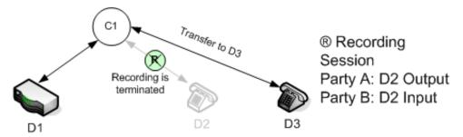
When the call is transferred to D3, the Recording Session is maintained and should expect a reINVITE to re-negotiate the media between D1 and D3. The media control dialog between SIP Server and Media Server is also maintained by only sending reINVITEs to the media control dialog.
