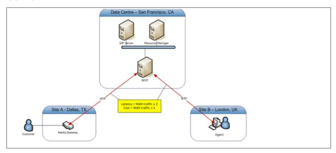
When the Media Control Platform (MCP) is located at the data center site, the deployment needs to double the WAN traffic because the media path needs to be bridged through the data center. This increased WAN traffic leads to increased latency of the media path by doubling the WAN path.
