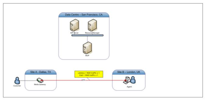
In a typical scenario, the customer might be calling into a contact center site with a media gateway, and the agent is located in a different site from the media gateway.
