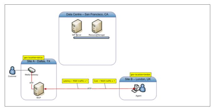
To minimize latency, the geo-location feature has been introduced in SIP Server and Resource Manager. This feature allows MCPs to be deployed in a remote site that is close to one of the parties in the call. This diagram is a deployment that places MCP in Dallas as set in the geo-location=dallas parameter.
