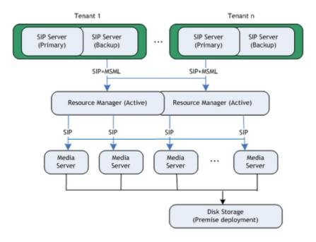
A media server (MCP) cluster is managed by a pair of Resource Managers running in Active-Active mode. Resource Manager identifies the tenant coming from SIP Server and selects the appropriate IVR Profile for the call. Each MCP instance in the cluster is able to handle call recording for any tenant based on the IVR Profile information.
