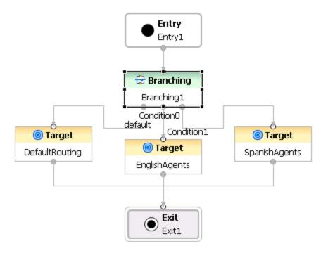
It uses drag-and-drop to arrange, add, and delete blocks on a design area. The blocks are connected within the design area to build the flow for the application. You define the properties for a selected block in Composer's *Properties view*. Also see: Working With Diagram Layouts
