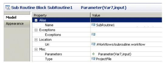
Now the Parameters property can be used for the Parameter Synchronization. The main diagram implicitly parses the sub-workflow parameters and lists them in the Parameter settings dialog as shown below.
