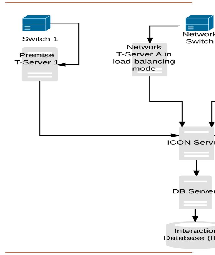
Multiple T-Servers per ICON-IDB Pair Deployment: Multiple Network T-Servers per Switch (Load-Balancing Configuration)
