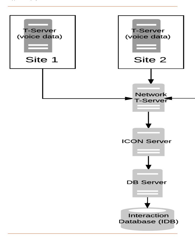
Network Deployment: A Single Network T-Server per Network Switch
