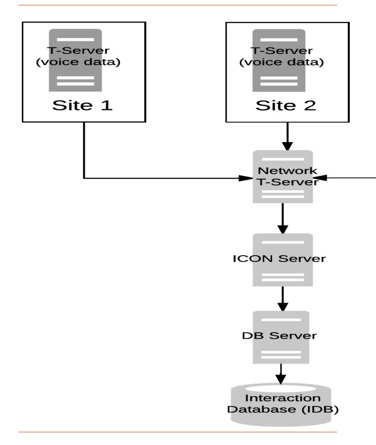
Network Deployment: A Single Network T-Server per Network Switch
