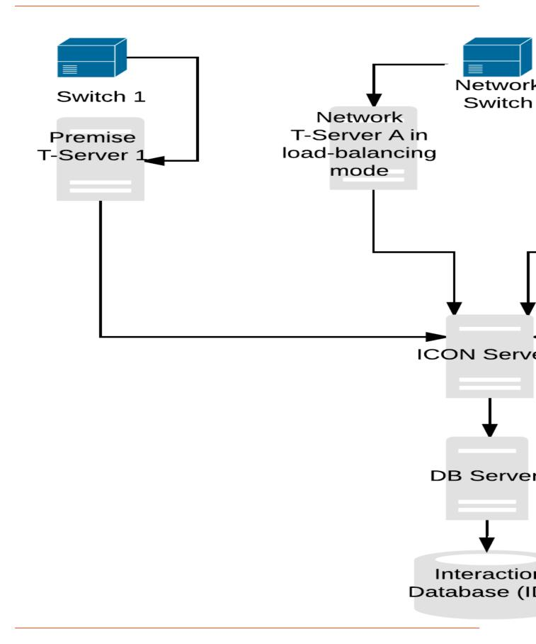
Multiple T-Servers per ICON-IDB Pair Deployment: Multiple Network T-Servers per Switch (Load-Balancing Configuration)
