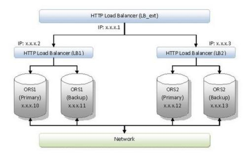
In the above diagram, ORS1 (both Primary and Backup servers) will have the address of ORS1 HTTP Load Balancer configured as the external-url. Similarly, the ORS2 will have ORS2 HTTP Load Balancer configured as its external-url. The load balancers will distribute HTTP requests across all ORS Nodes in the cluster and the ORS Nodes will automatically ensure that all requests corresponding to one session will be delivered to the correct Node.
