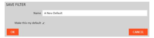
The **Save Filter** dialog allows a user to save a new filter or edit an existing one. Each filters name must be unique and if a filter with is saved using an existing filters name then it will replace it. If **Make this my default** is checked then this will also make the selected filter the default for the page.
