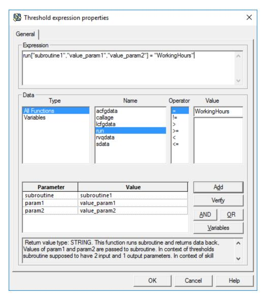
When accessing function from skill expression, IRD shows only subroutines that have 4 input and 1 output parameters.
