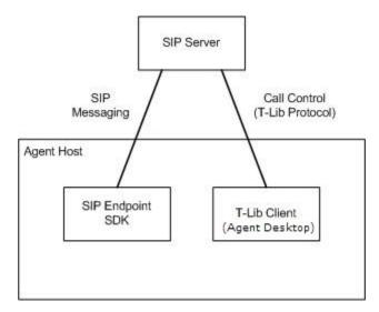
As you can see, the SIP Endpoint SDK handles the SIP messaging, and the T-Lib Client (Agent Desktop) uses the T-Lib protocol to handle call control.
